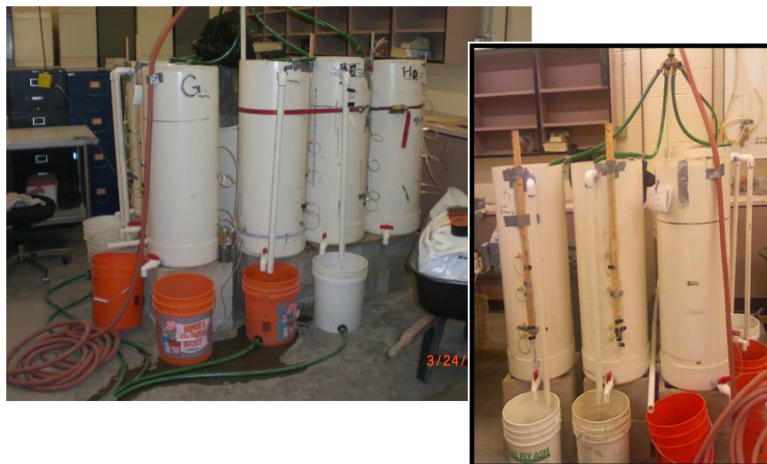
Laboratory Tests on Soil Mix and Infiltration Rate Infiltration Rate = fct (Mix of Sand, Soil, Others etc, and Clogging Effect)
