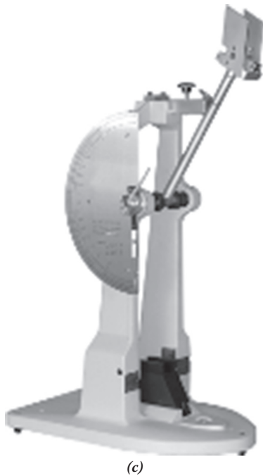
Figure 2-11 Impact testing devices and equipment: (a) Izod test specimen and striker (side view), (b) Charpy test specimen and striker (top view), (c) pendulum-type impact tester, and (d) drop-type impact tester. (Courtesy of Instron Corporation, Norwood, MA.)
