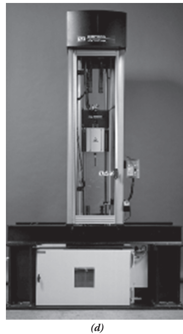
Figure 2-11 Impact testing devices and equipment: (a) Izod test specimen and striker (side view), (b) Charpy test specimen and striker (top view), (c) pendulum-type impact tester, and (d) drop-type impact tester. (Courtesy of Instron Corporation, Norwood, MA.)
